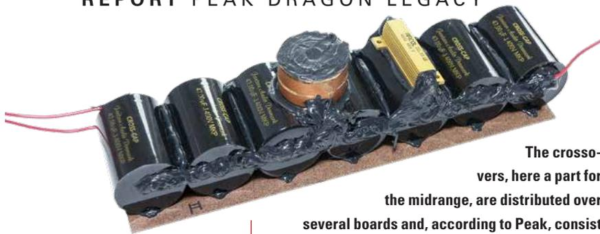
**The crossovers, here a part for the midrange, are distributed over several boards and, according to Peak, consist of the highest quality components available.**
