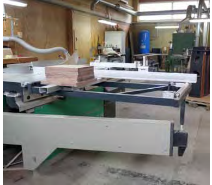
The huge, flat-bed saw bench that is used to cut panels for lamination.
