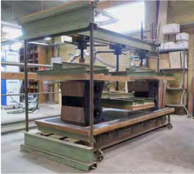
A serious linear router, perfect for machining channels or bevels into cabinet panels.
