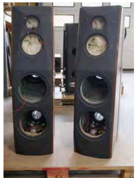
A pair of El Diablo cabinets awaiting their crossovers. Even a cabinet this substantial still needs to control the internal air mass
