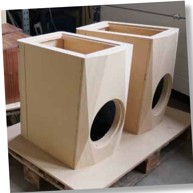
Lower bass cabinets for the Dragão Legacy in raw form: look carefully at the baffle and you can see the contour lines of the HDF laminations.
