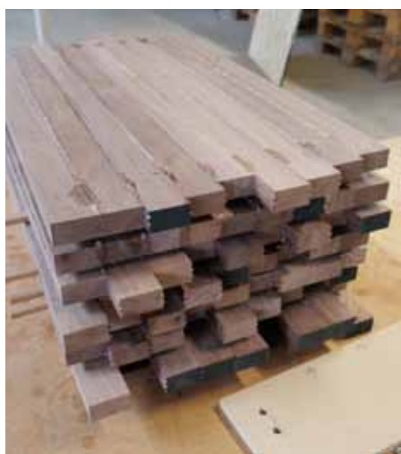
Bonded hardwood strips. Note the staggered arrangement that helps match grain and figuring.
