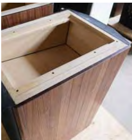
Closer view of the almost finished cabinet with front and rear 'leather' and hardwood skin. Note the sloping internal baffle, creating a non-parallel enclosure (mirrored by the slope on the top of the cabinet).
