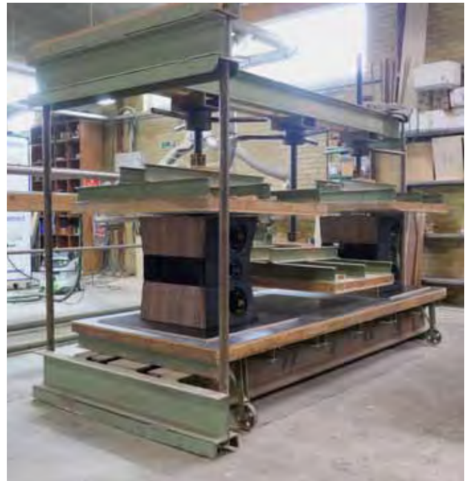
Some processes need more than just clamping! The massive presses used to bond elements of the Dragon Legacy together.
