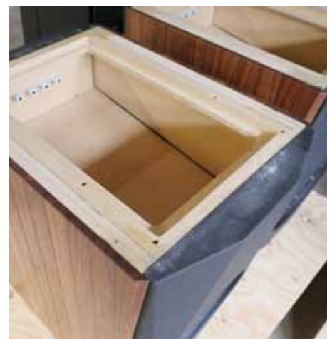
Note the terminals in the rear face of this separate section of the enclosure. It will house the crossover and be filled with sand for added damping before sealing.
